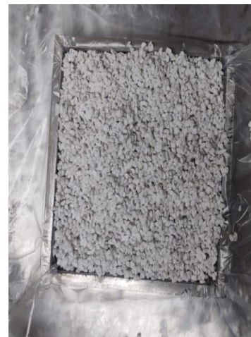
(c) Placing the core up on the lower skin
