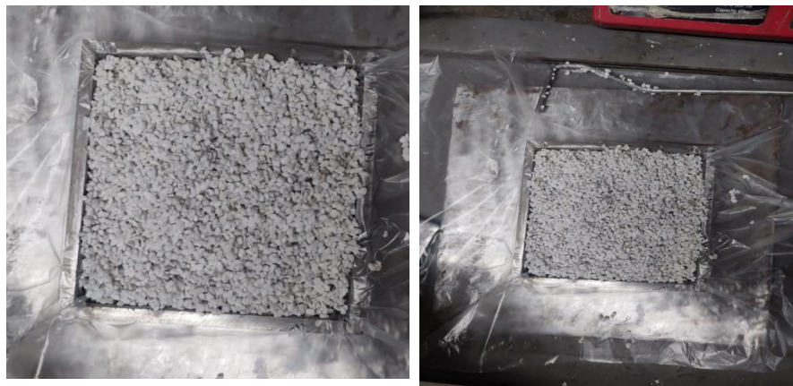
(b) Pouring perlite mixture inside the mold (c) Prepared core
