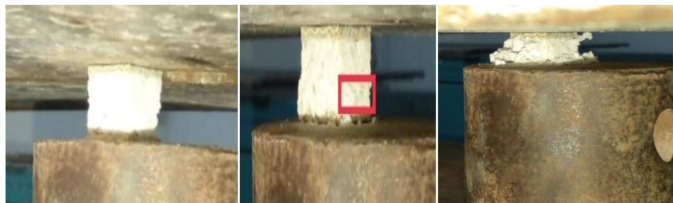
(a) Initial (b) Start de-bonding core (c) Final Failure
