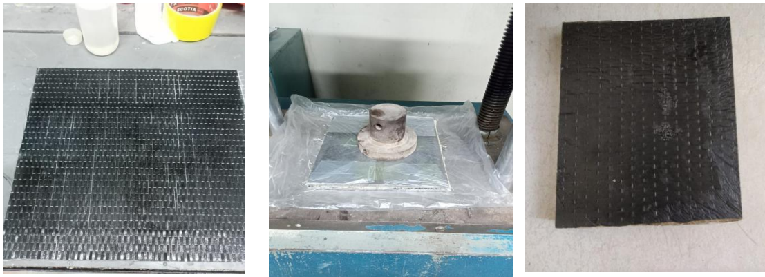
(d)Placing the upper skin (e)Compression process (f)Fabricated Sandwich Composites
