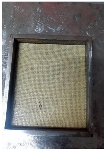
(b) Placing the skin into the mold
