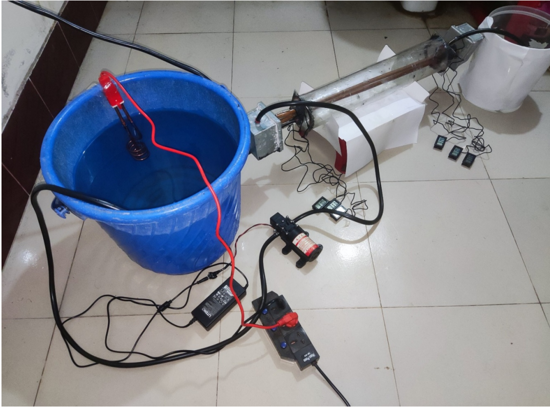
Figure 3.16: Experimental Setup of Straight Tube Heat exchanger
