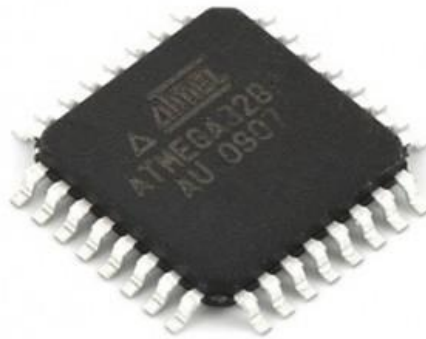
Figure 3.3: Micro controller IC AT Mega 328p
