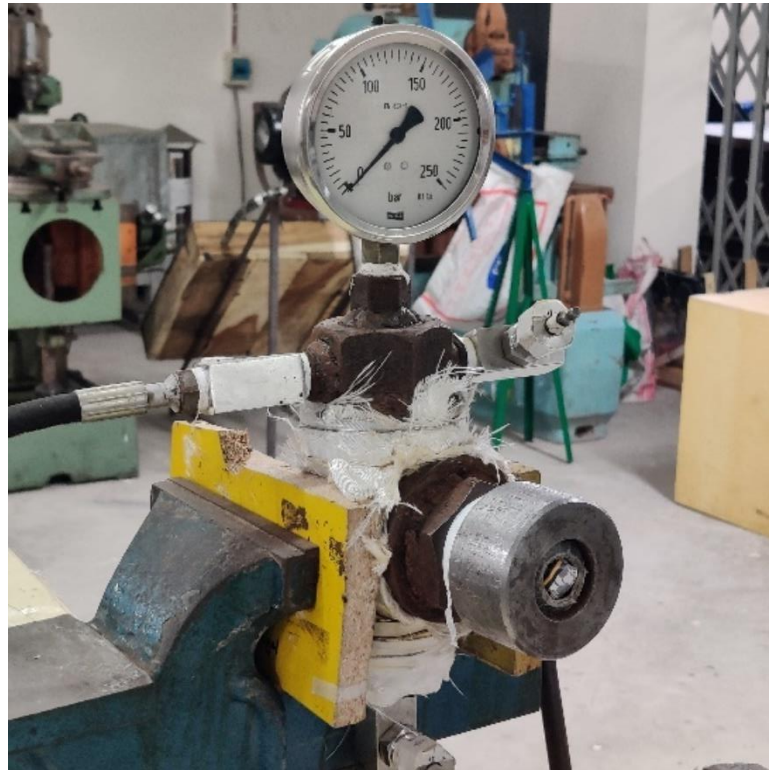
Figure 9: Installation of supercritical dryer (autoclave)
