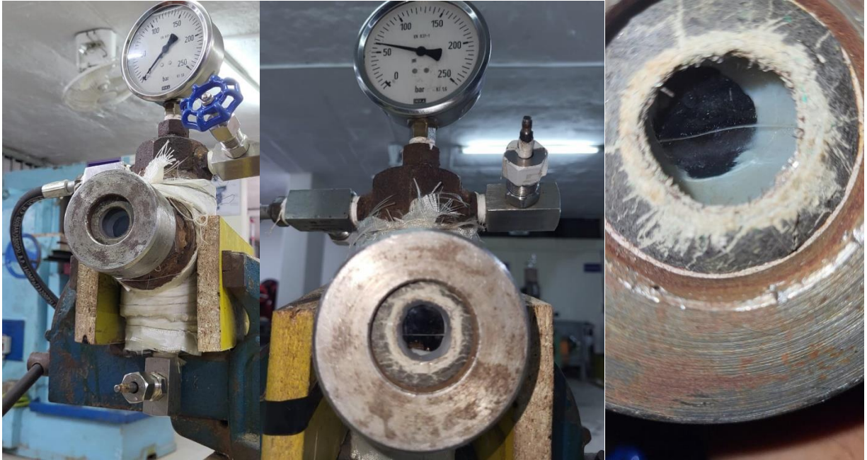
Figure 19: Filling with Supercritical Fluid
