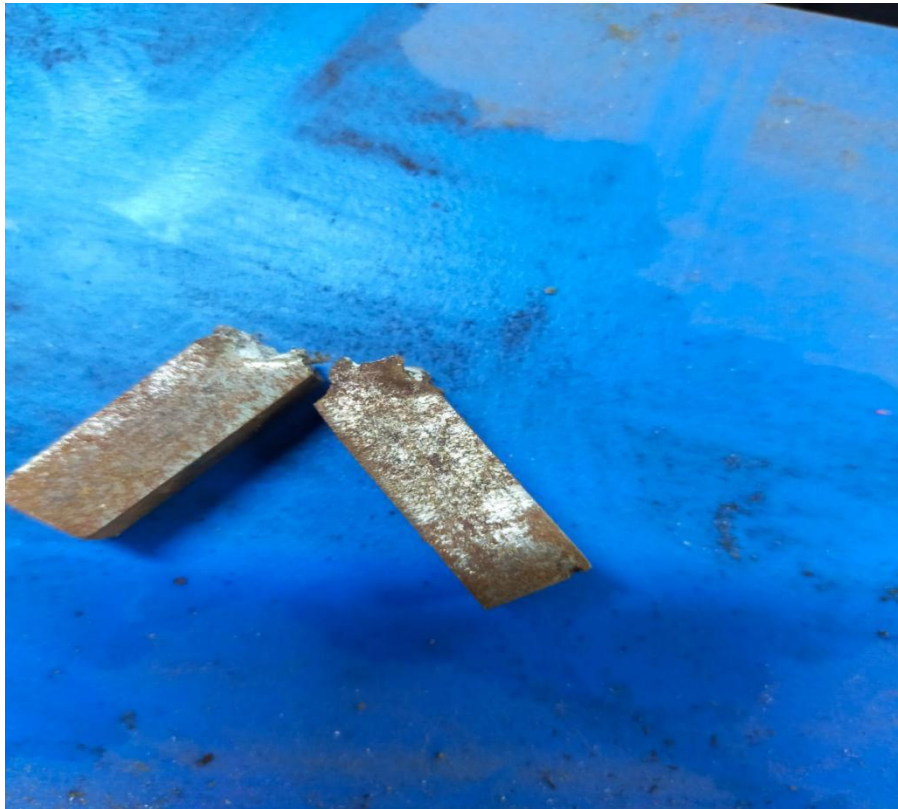
Fig5.6: Breaking after Impact test (TIG)
