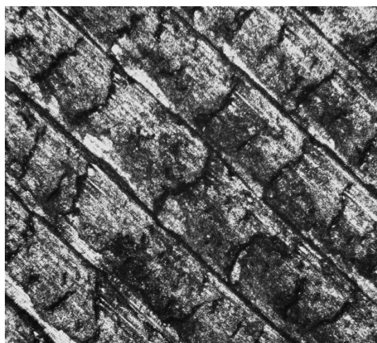
Fig: TIG welded zone at interfaces: -10x
