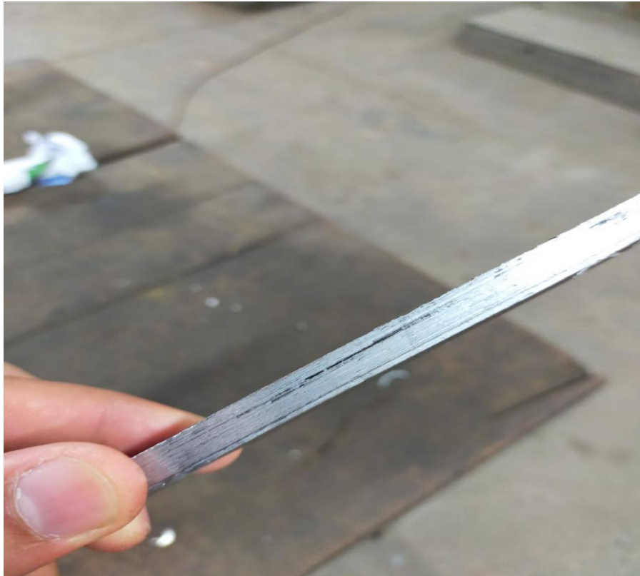
Fig10.2: Prepared 12.50 mm thickness sample from Side bend test
