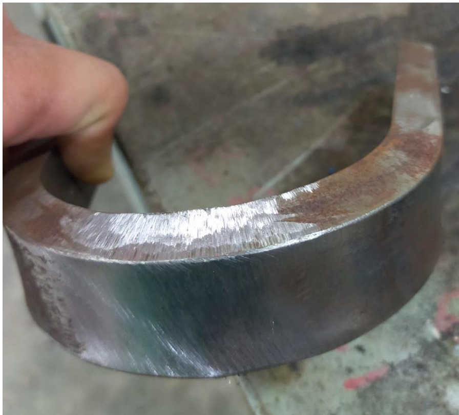
Fig8.3: After Face Bending test (Arc)
