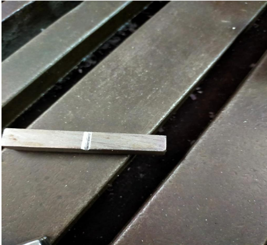
Fig5.3:45° angle Sample ready for Impact Test by Milling Machine
