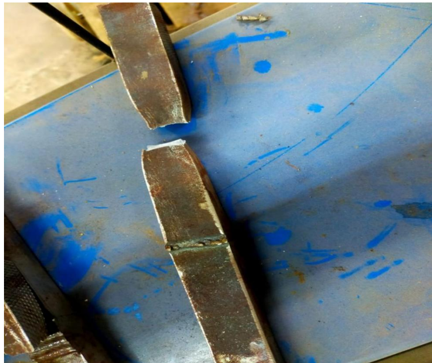
Fig4.3: Breaking Base metal zone(TIG)
