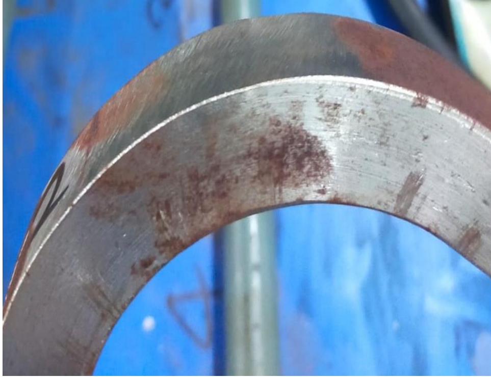
Fig10.4: After Side Bending test
