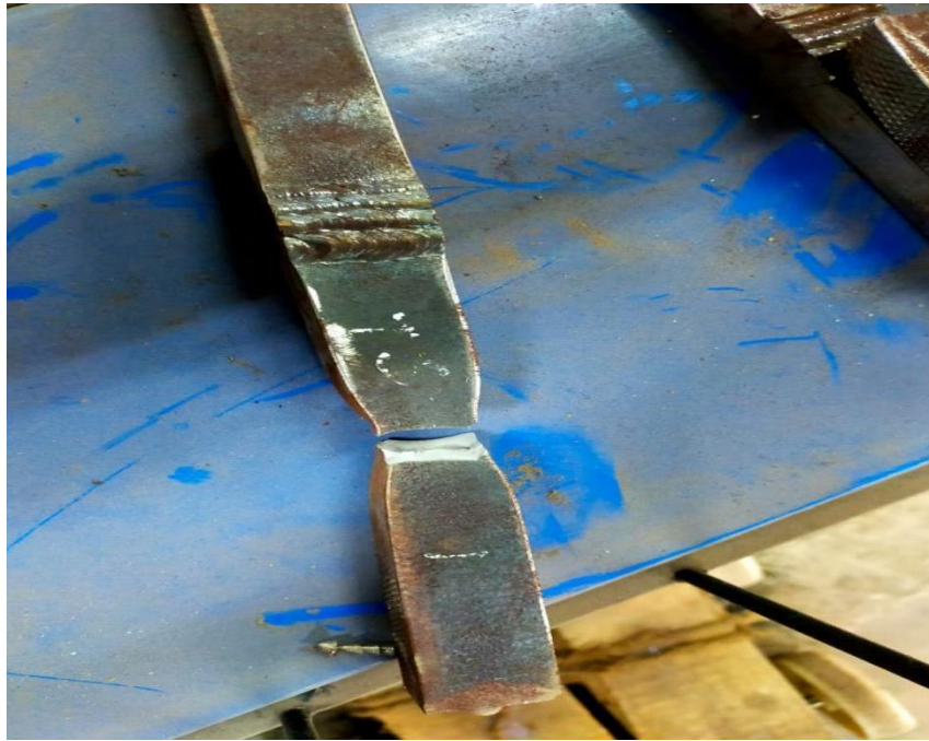
Fig4.5: Breaking Base metal zone (Arc)
