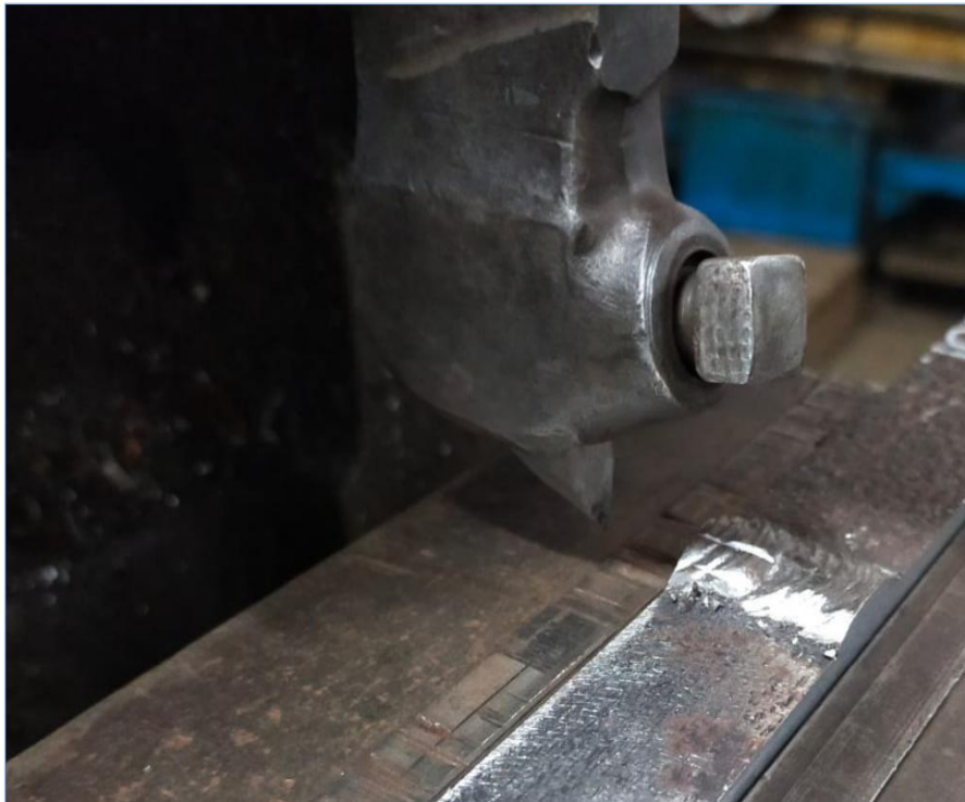
Fig8.1: Face zone cutting by Shaper Machine
