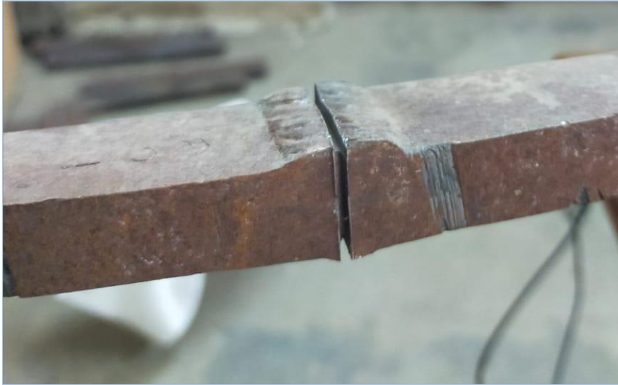
Fig6.3: Slot Cutting sample for braking
