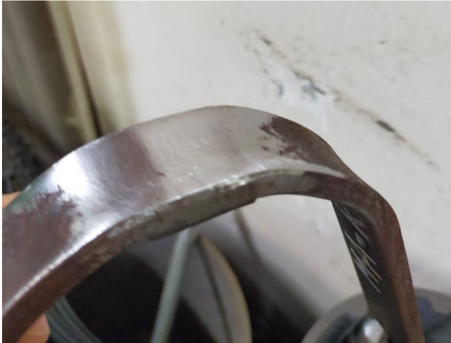
Fig 9.4: After Root Bending test (TIG)
