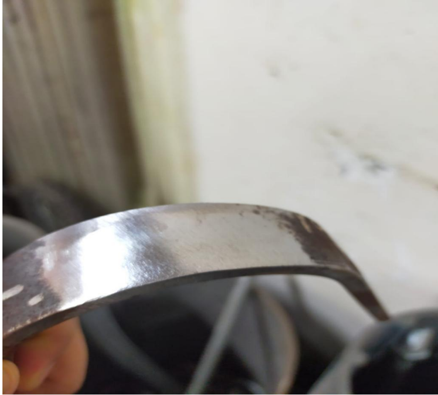
Fig8.4: After Face Bending test (TIG)
