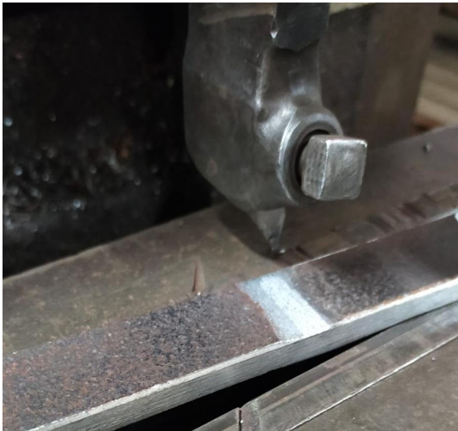
Fig9.1: Root zone cutting by Shaper Machine
