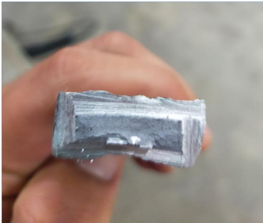
Fig6.6: No crack is found (TIG welding joint)
