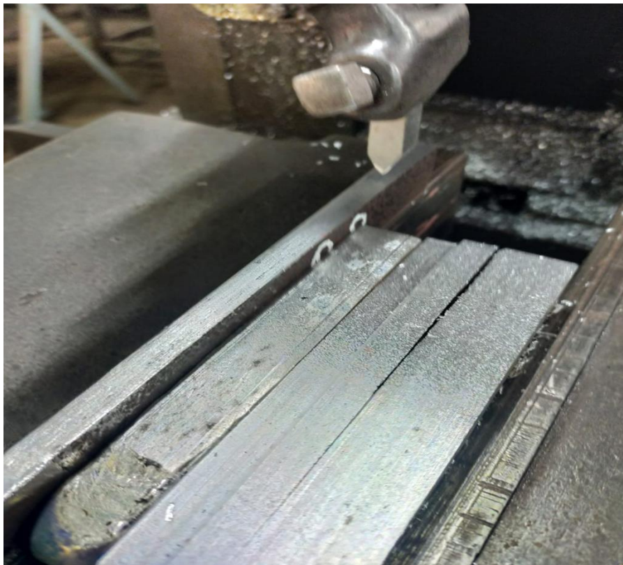
Fig 10.1: Reducing wide side zone cutting by Shaper Machine
