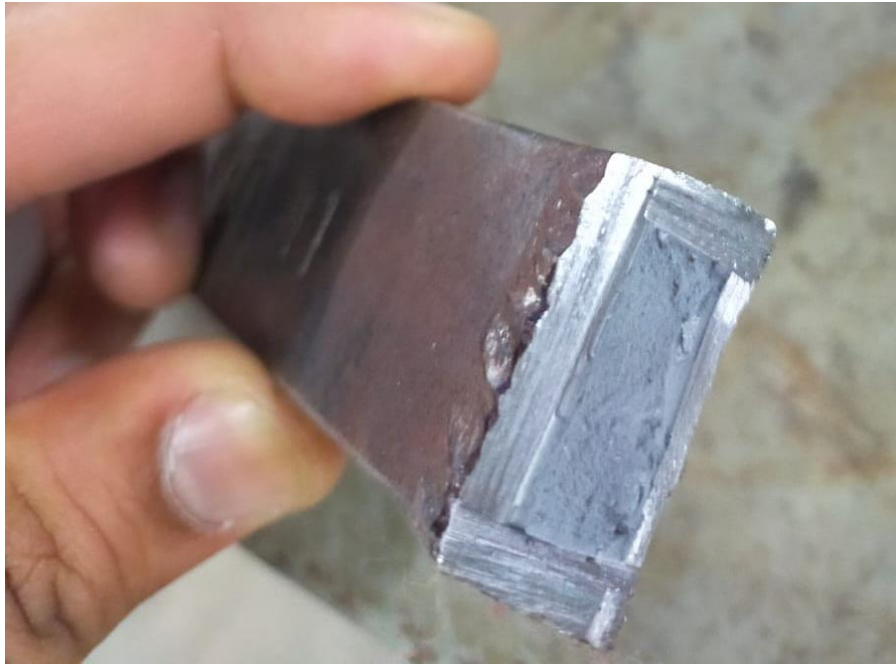
Fig6.5: No crack is found (Arc welding joint)
