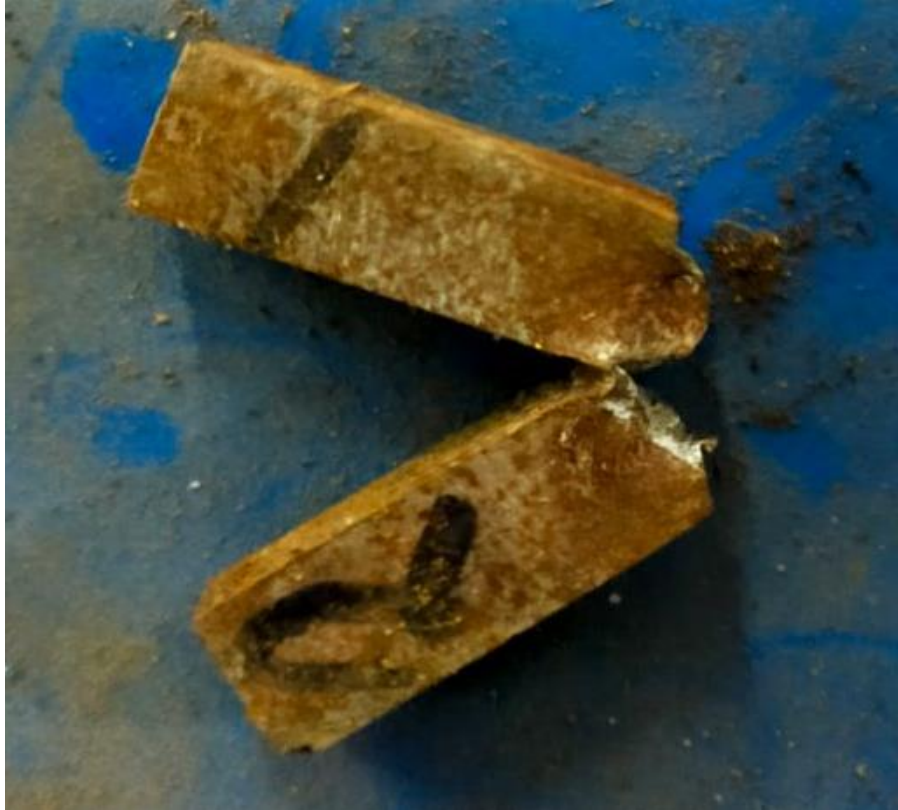
Fig5.5: Breaking after Impact test (Arc)
