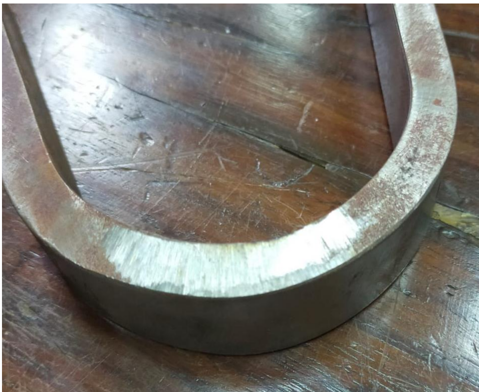
Fig 9.3: After Root Bending test (Arc)
