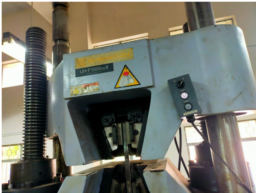
Fig6.4: Holding Sample for Nick break
