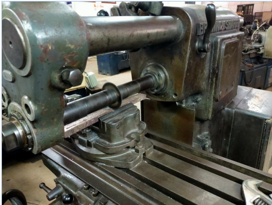
Fig6.2: Milling Machine cutting with slitting saw cutter in Welded Face zone
