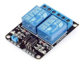
Figure 3.16: Relay Module
