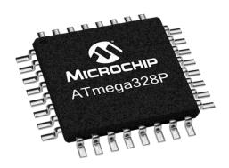
Figure 3.6: Micro-controller IC AT mega 328p.
