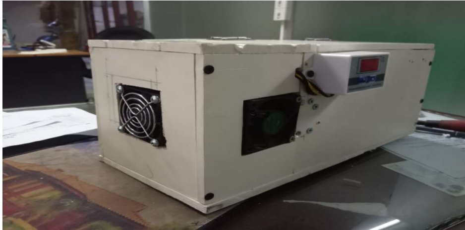
Fig.4:1 Construction of Potable Refrigerant Unit
