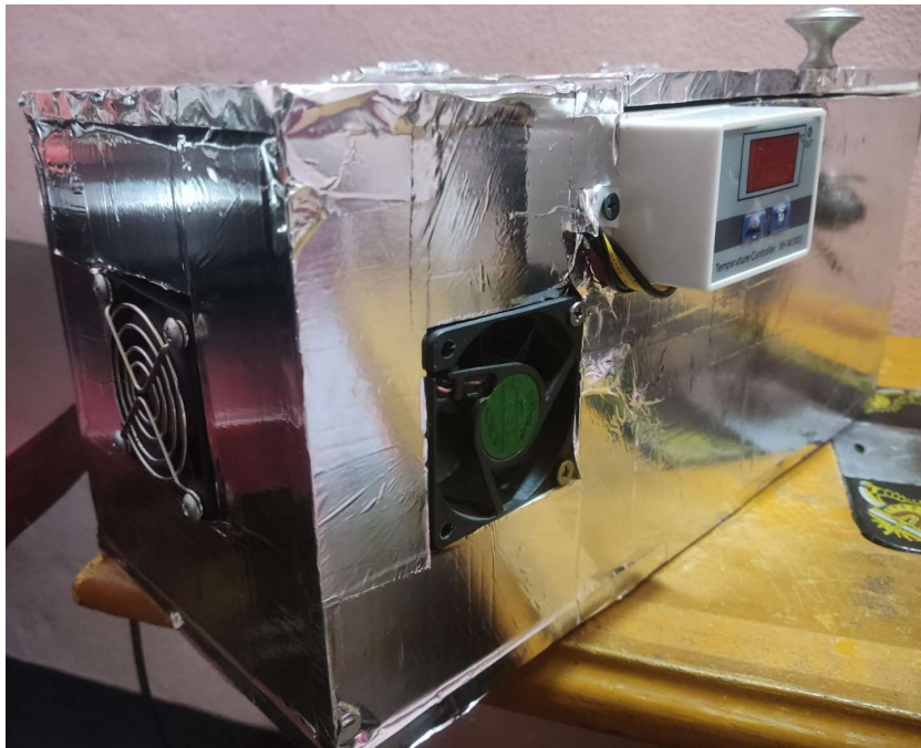
Fig.4:2 Construction of Potable Refrigerant Unit
