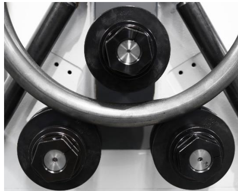
Fig:2.7 Hydraulic Profile Bending
