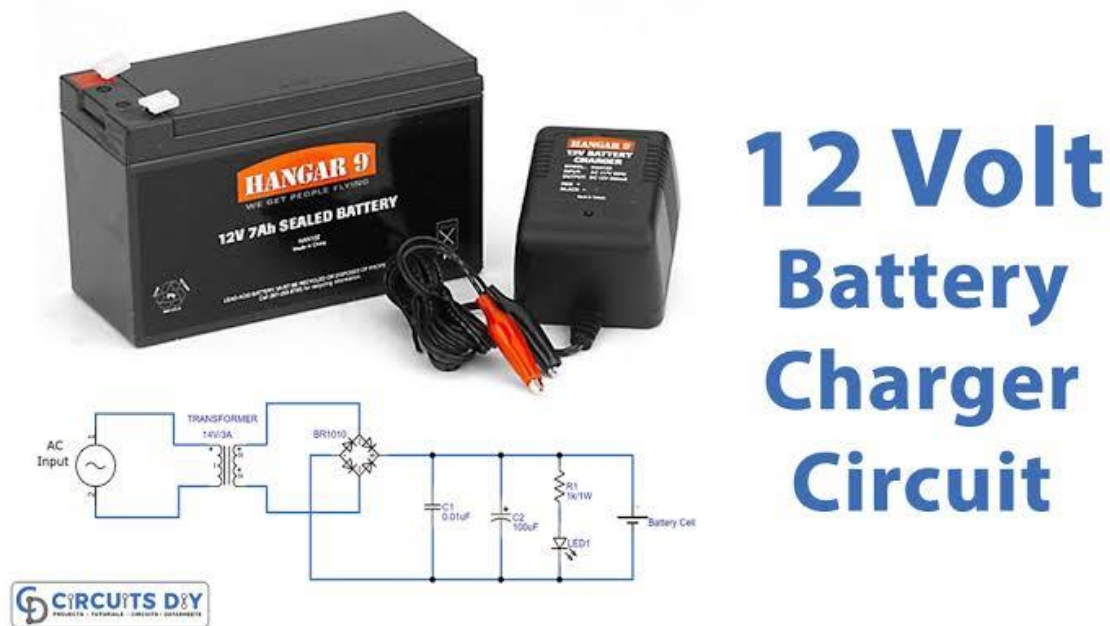
Fig 3 : 12 volt Battery charger circuit
