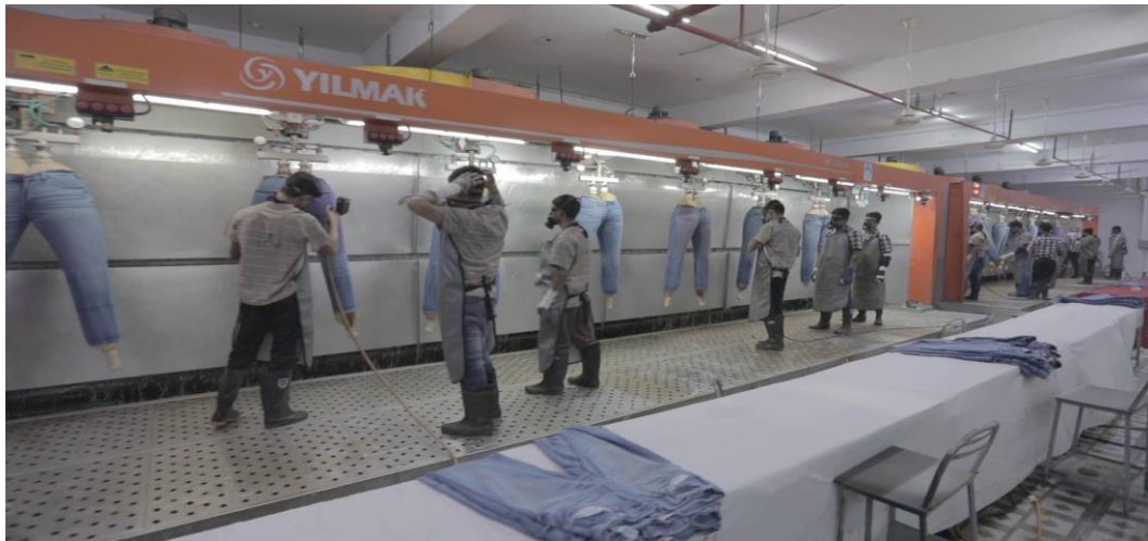
Fig: Dry Process (Spraying)
