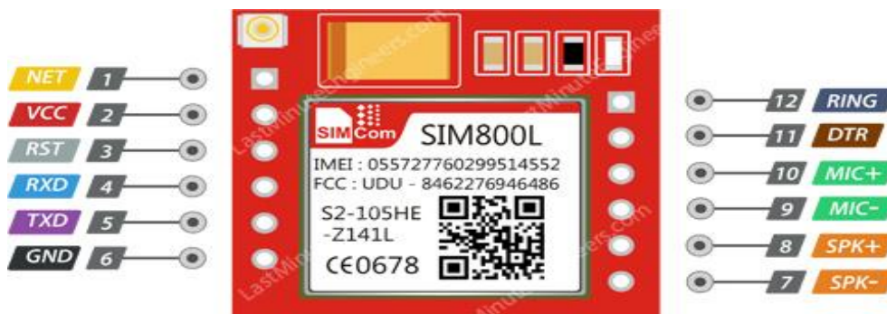
Figure 3.14: GSM Module Pinout
