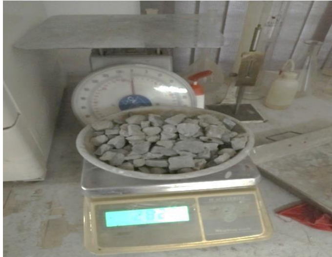
Figure No: 3.1 Weighing Test Sample in Saturated Surface-Dry Condition
