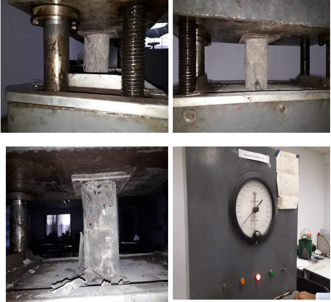
Figure No: 3.16 Cylinder Testing on UTM
