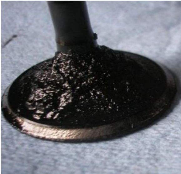
Fig.4.19: Carbon buildup on engine valve.
