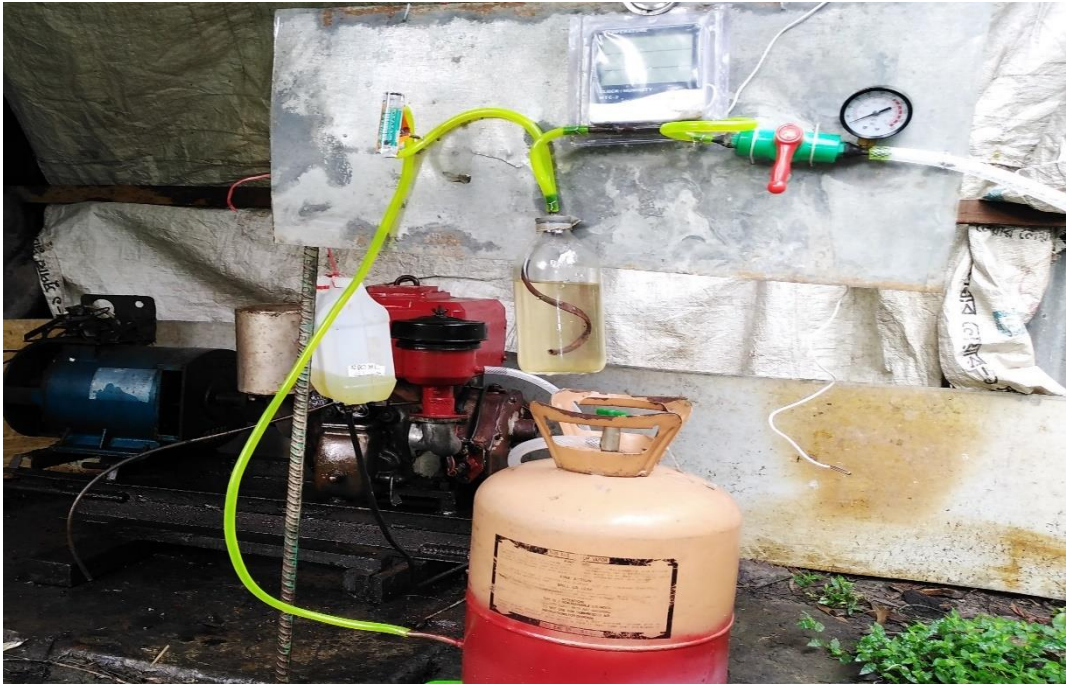
Fig.4.11: Dual fuel Setup Project picture.
