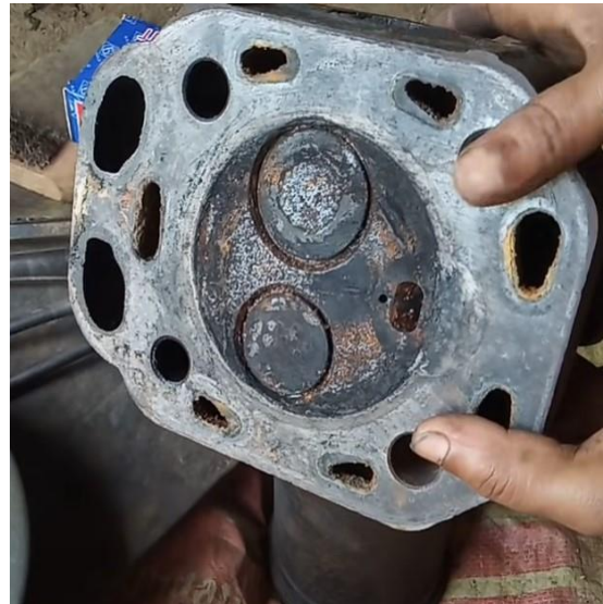
Fig.4.20: Carbon buildup on head.
