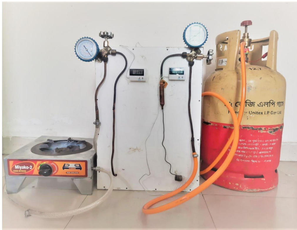
Fig:3.6 Construction Diagram of LPG Refrigerator
