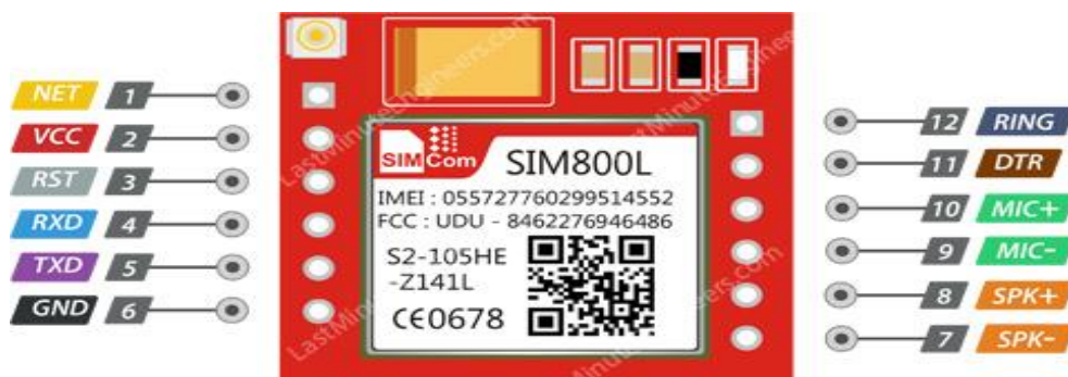
Figure 2.17: GSM Module Pinout
