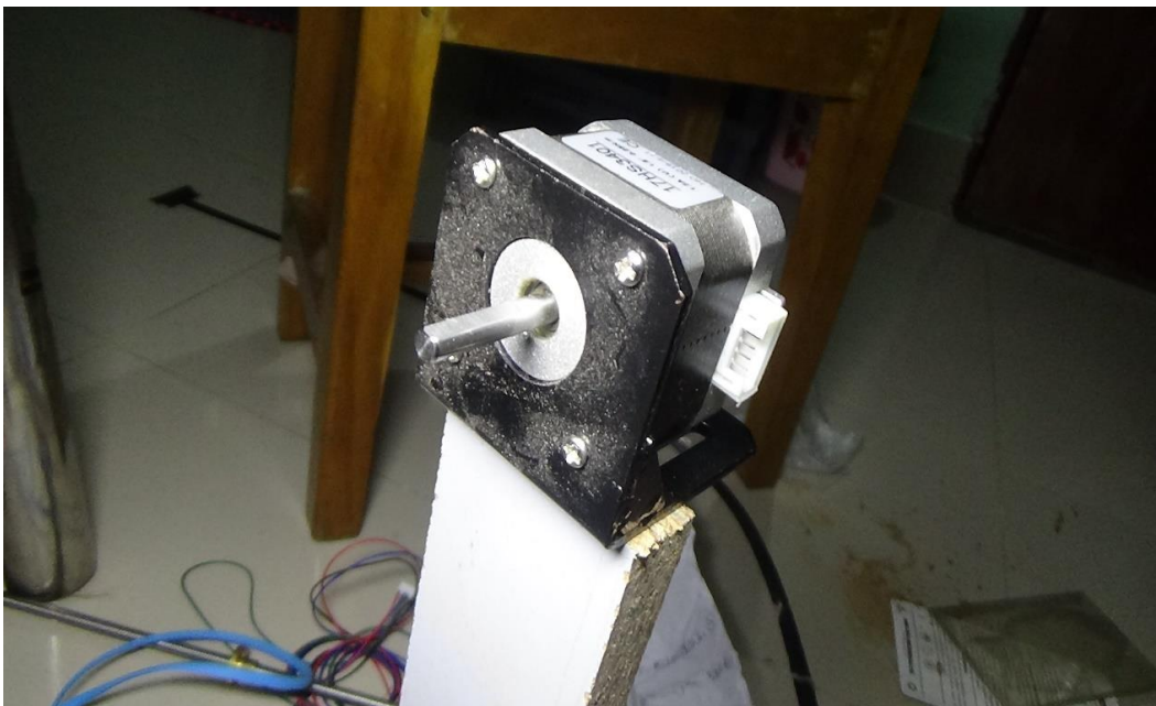
Figure 3.33: L shape angle installed with motor
