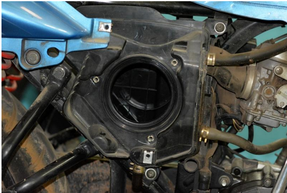
Fig2: Installation position of non conventional supercharger.
