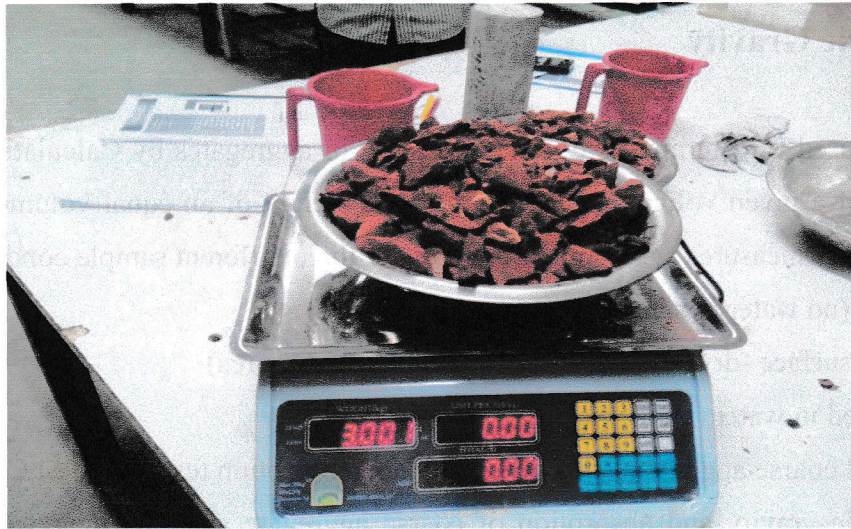
Figure 3.1 Measurement of brick chips
