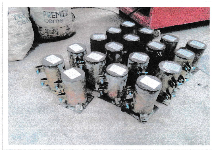
Figure 3.5 Casting of concrete cylinder
