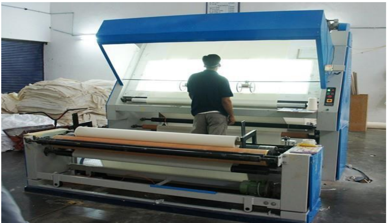
Figure: Fabric inspection
