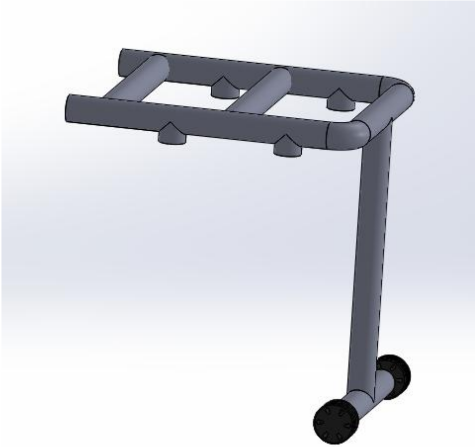
Figure 5.5.7: 3D Figure Of Main Frame With Wheel.
