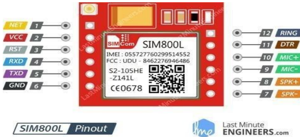
Figure 7:GSM Module Pin out
